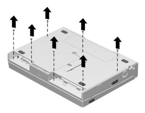
Figure 5-37. Removing the Keyboard Screws
